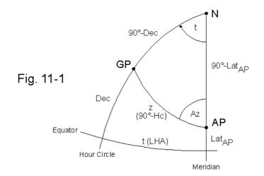
When using the intercept method, the latitude of the assumed position,  $Lat_{AP}$ , the declination of the observed celestial body, Dec, and the meridian angle, t, or the local hour angle, LHA, (calculated from the longitude of AP and the GHA of the object), are initially known to the observer.
