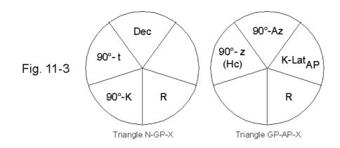
According to Napier's rules, Hc and Az are calculated by means of the following formulas:
