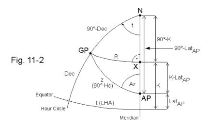
The first right triangle is formed by GP, N, and X, the second one by GP, X, and AP. The **auxiliary parts** R and K are intermediate quantities used to calculate z (or Hc) and Az. K is the angular distance of X from the equator, measured through AP. Both triangles are solved using **Napier's Rules of Circular Parts** (see chapter 9). *Fig. 11-3* illustrates the corresponding circular diagrams:
